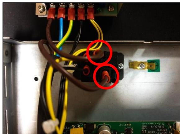
You can now use a 5.5mm nut spinner or spanner to remove the nut securing the earth bond in place as pictured below, left. Once the nut is removed, the earth bond is free.
