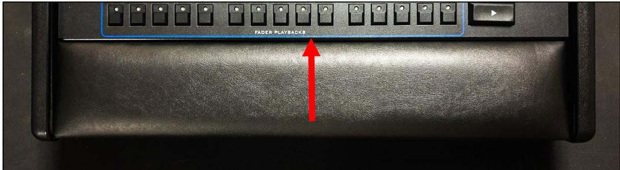
Once the arm rest has been removed, you will have access to all screws securing the front panel assembly in place. Remove 14x M3x6 black countersunk screws from the locations pictured below using a PZ1 screwdriver. These screws can now be discarded.
