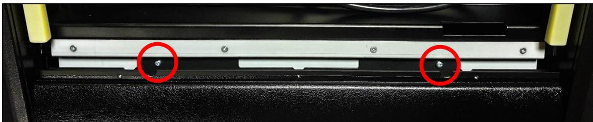
Next, carefully place the back end of the new MQ500M Wing front panel onto the chassis at roughly a 45-degree angle. While holding the panel up, reconnect the front panel cable and earth bond as previously removed from the old front panel assembly. Once these are connected, you can then also connect the power supply cable for the motorised faders. Note that this cable has a tight fit, and you may need to lower the front panel further to connect it. See both images on the next page for reference.
