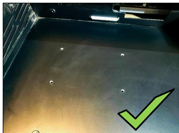
Once the area is clean, lift the wing from the front and file out the holes from the underside so they are smooth, and screws will comfortably fit through. The image to the right shows the drill holes from the underside of the wing, before being filed out. Once the holes are filed and any new metal shavings are removed, you are ready to screw in the new power supply.
